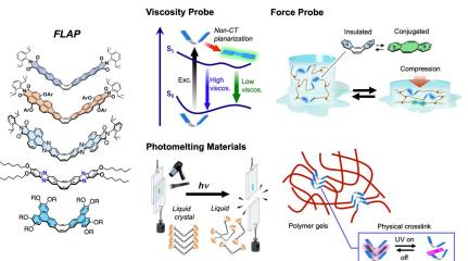
**3)** Photomelting materials: Twofold  $\pi$ -stacking of V-shaped molecules exhibits high cohesive force of materials, while excited-state planarization plays a key role for photoinduced melting. The control of assembly develops light-melt adhesives and photomelting gels on demand.
